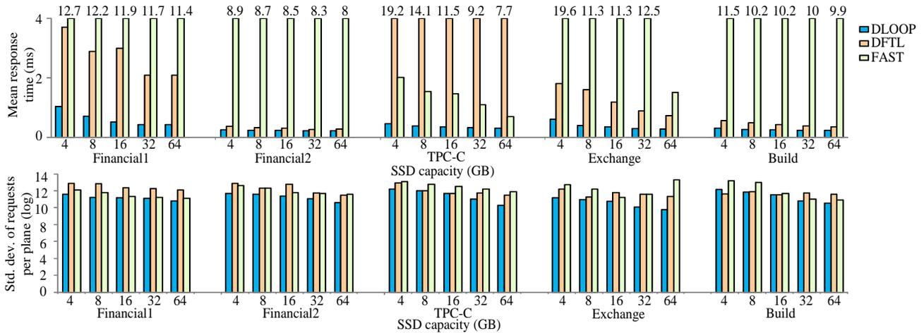
Figure 8. The impacts of flash SSD capacity
