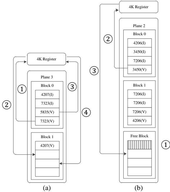
Figure 5. Merge operations in DLOOP
