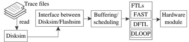
Figure 7. Architecture of the extended simulator
