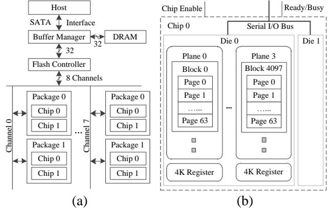
Figure 1. (a) Flash SSD block diagram; (b) internal chip structure
