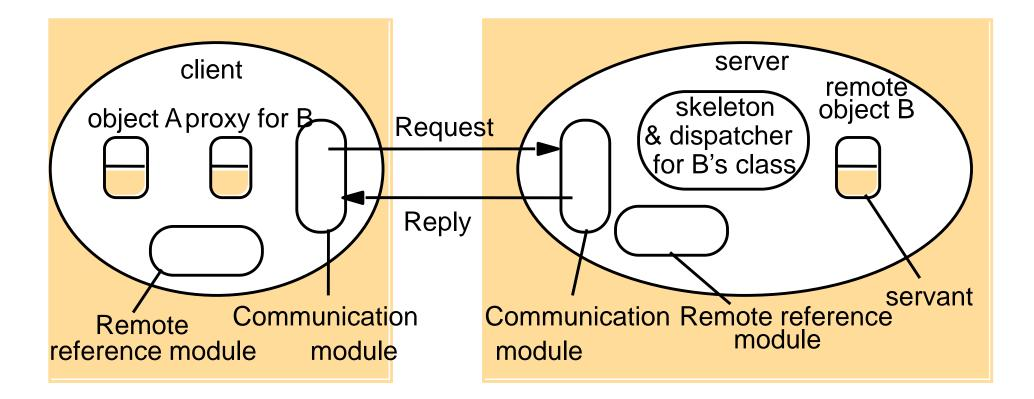
**Communication Module is** Responsible for communicating messages (requests and replies) between the client and the server. It uses three fields from the message:
