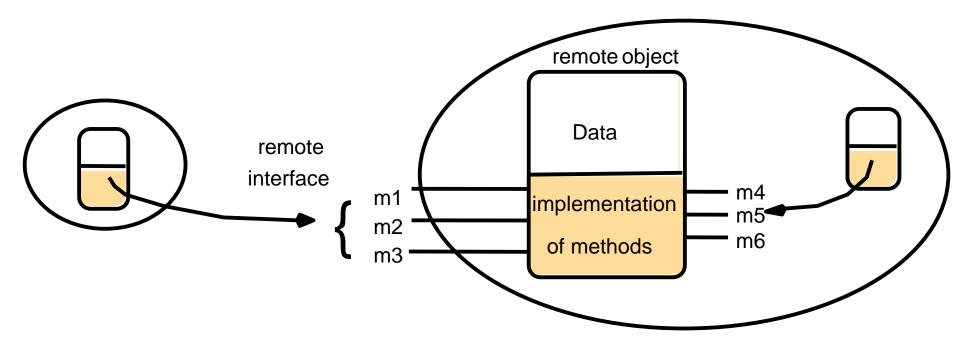
The class of a remote object implements the methods of its remote interface.
