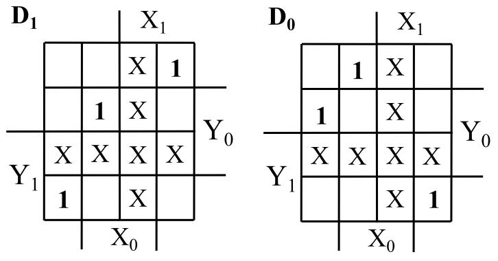
•  $\mathbf{D}_1 = Y_1 X_1' X_0' + Y_0 X_0 + Y_1' Y_0' X_1$ •  $\mathbf{D}_0 = Y_0 X_1' X_0' + Y_1 X_1 + Y_1' Y_0' X_0$
